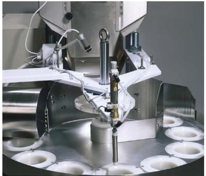
The product storage hopper with vibrating exit and level control feeds regularly a carousel of cups, made of special material for foodstuff industry, rotating on a lower plate. Volume can be controlled accordingly to product density with adjustable telescopic dosing cups. When different weights are required, special additional reductions will fit allowing different dosing volumes with the same machine.
